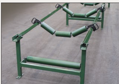
Complete Canning Field Conveyor Bay (750mm belt - polymer safety handles - in 3.048m long bays).
